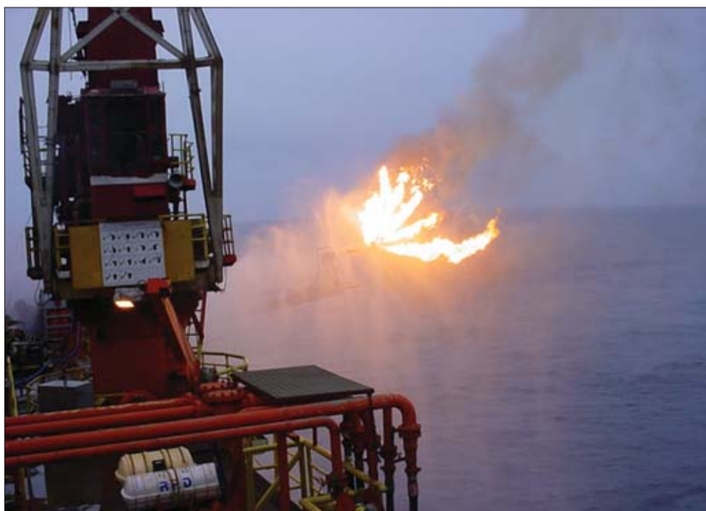
Photo of the initial flare whilst testing the 4 Athena Discovery. To test a well they produce the oil to determine the flow rate and burn it through a flare rather than collect it.
